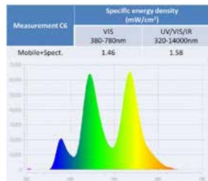
Visible part of the light spectrum of laptop LCD screen recorded without filters and the same light spectrum recorded through nanophotonic glasses. Significant difference in the reduction of total spectrum by 56% and the most in the case of blue spectrum, with a relative increase of green spectrum.
