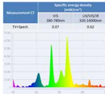
Visible part of the light spectrum of LED TV screen recorded without filters and the same light spectrum recorded through nanophotonic glasses. Significant difference in the reduction of total spectrum by 28% and the most in the case of blue spectrum, by 80%.
