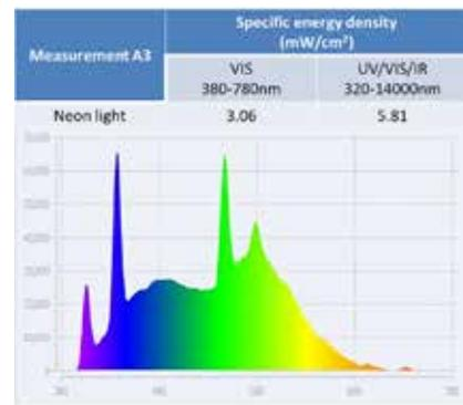
Visible part of the neon light spectrum recorded without filters and the same light spectrum recorded through nanophotonic glasses. Significant difference in the reduction of total spectrum by 58% and primarily UV and high-energy blue spectrum.
